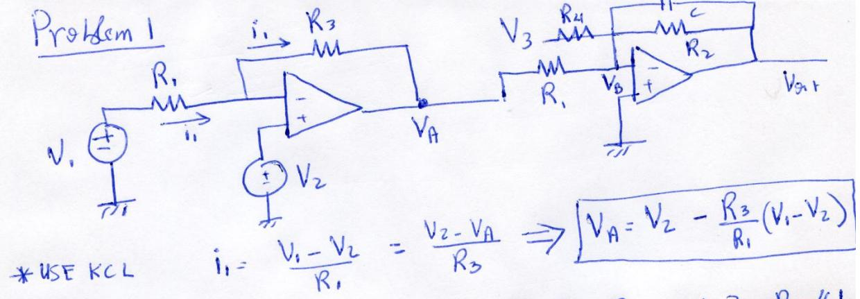
\* In second stage, we have inverting amp ~~with Z = R2~~. and ~~and Z = R2SC~~
