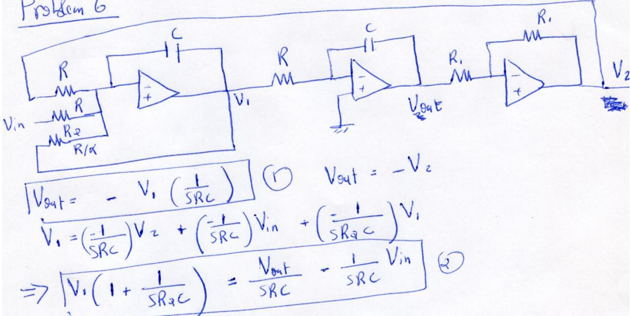
$$V_{out} = -V_1 \left( \frac{1}{SRC} \right) \quad (1) \quad V_{out} = -V_2$$
