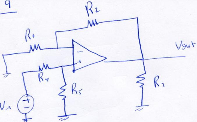
$$V^- = \frac{V_{out} R_1}{R_1 + R_2} = \frac{V_{out}}{9} \Rightarrow V_{out} = (V^+ - V^-) A_o(s)$$
